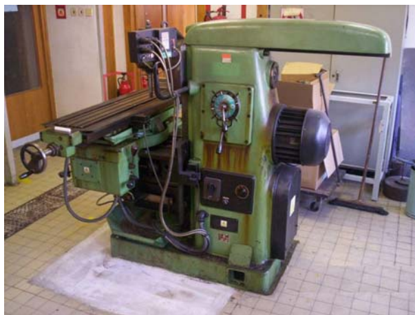
Figure 1: Tested milling machine with a vertical spindle — side view [3]
