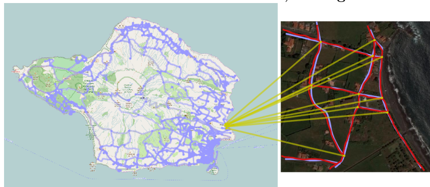
Figure 5.11: Examples of results for the roads dataset. On the left the graph extracted from the map is shown overlaid on a map image. On the right the graph extracted from the road network is shown (in red) aligned with the graph extracted from the map (in blue). The correspondences are depicted by the yellow lines connecting vertices of the graphs.
