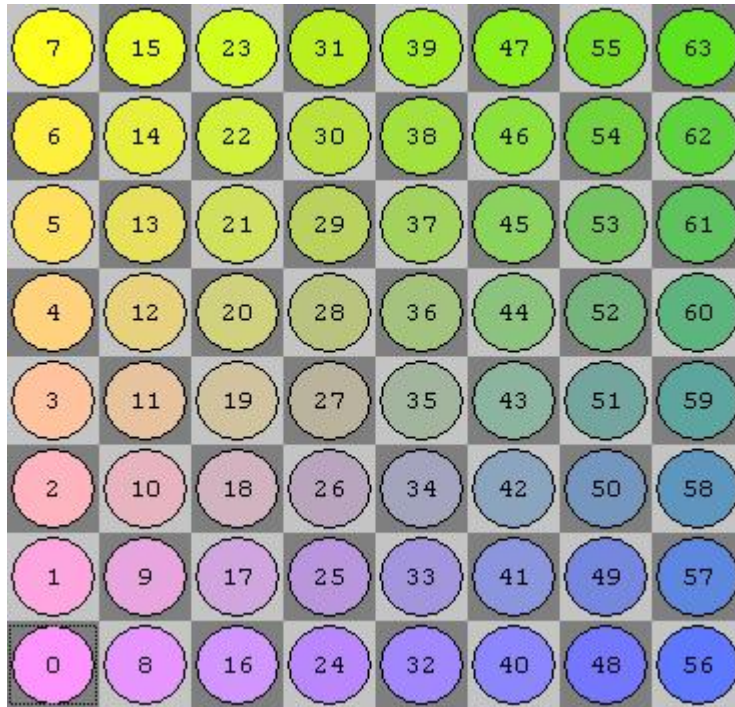
Figure 4.1: Bitboard representation by each bit [14]
