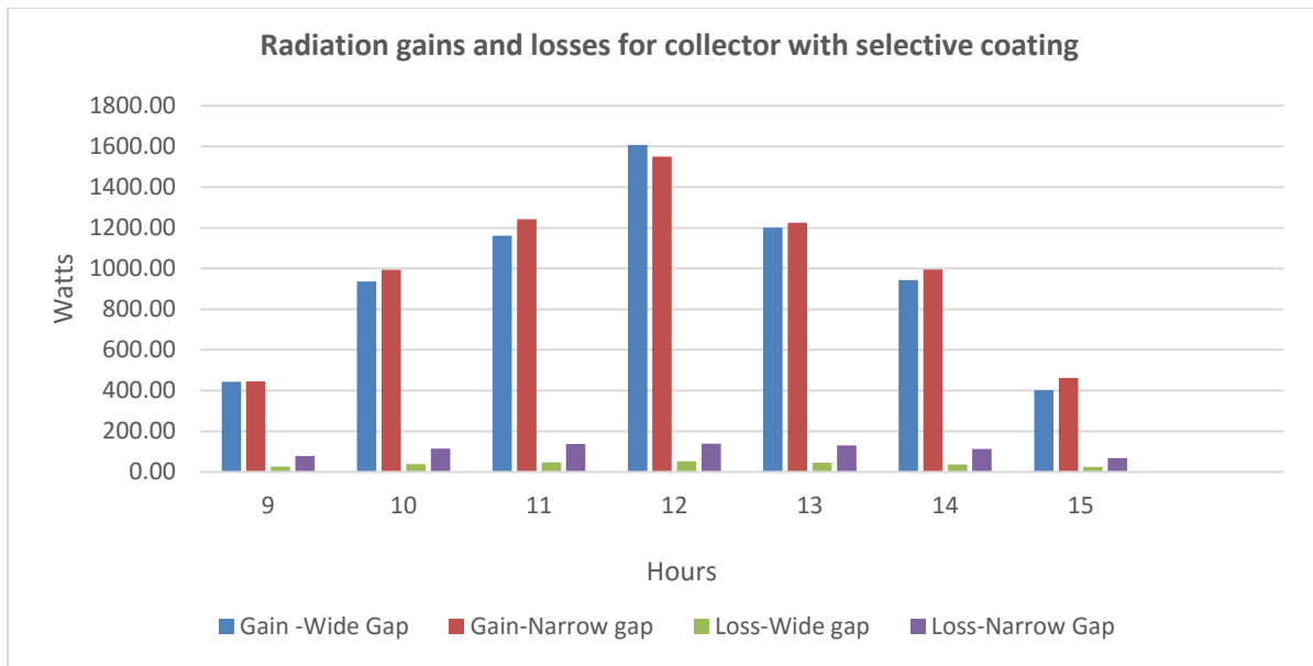
Figure 40 : Gains and losses for collectors with selective coating on 21 st December
