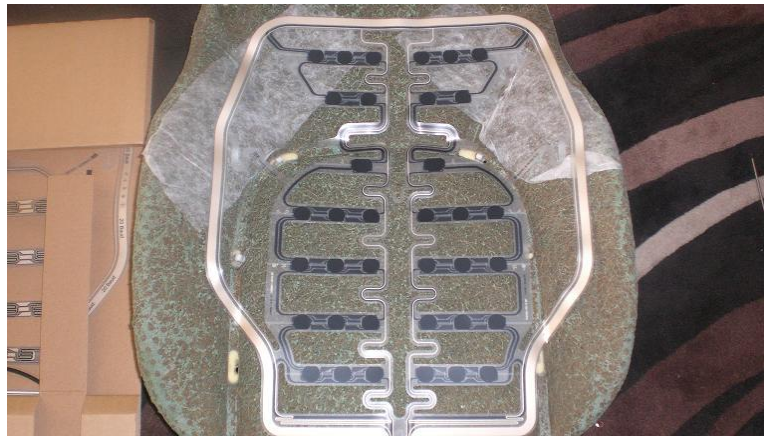
Pic. 4: Pressure seat sensor from Mercedes-Benz class A [8]
