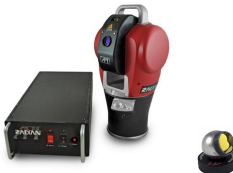
Obr. 1-9: Laser tracker API Radian, (zleva: kontrolér, laser tracker, SMR odražeč) [13]
