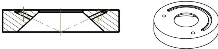
Figure 3.6: Weldment preform - bottom part
