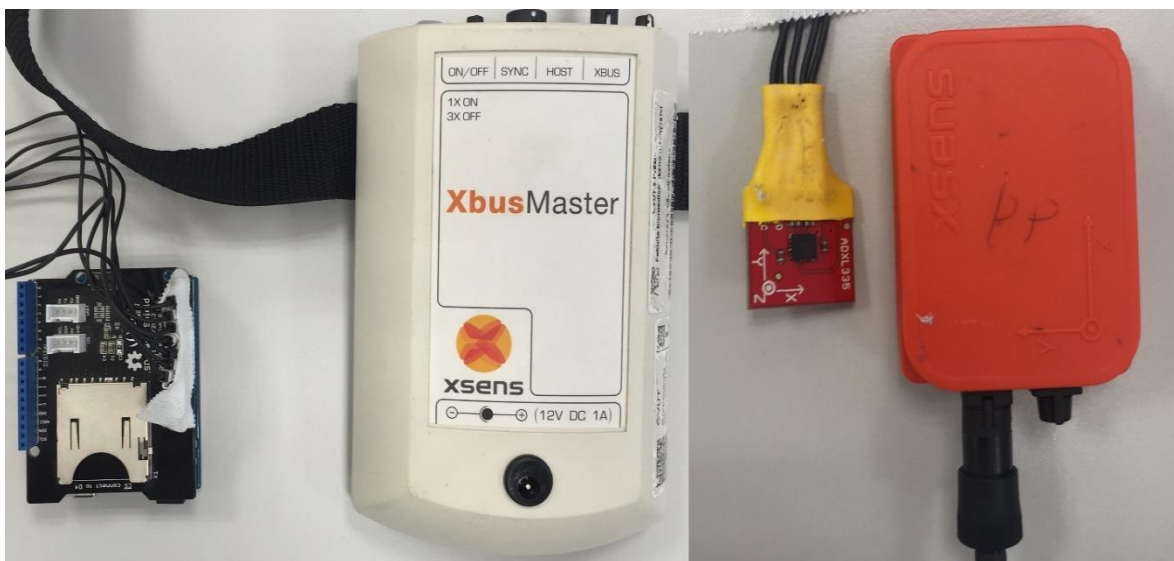
Fig. 34, size comparison of Xsens and our device based on Arduino board.
