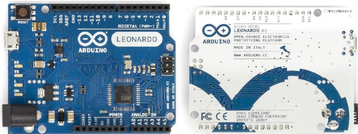
Fig. 15, Arduino Leonardo board, front and back side [27].
