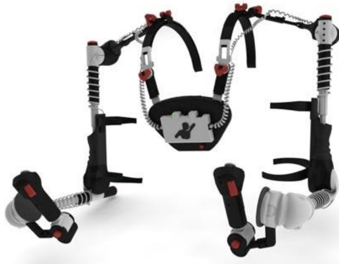
Fig. 11, mechanical motion capture system (exoskeleton) [13].
