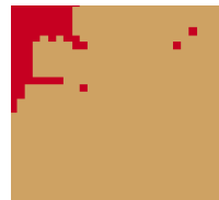
(b) The peninsula of the red domain is scissored and an orphan is created.
