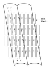
An arrangement such as shown this has several other advantages over simple pixel/lens parallel arrangement. The loss of resolution is distributed to both horizontal and vertical direction as opposed to full resolution in vertical direction and more severe loss in horizontal direction when vertical arrangement is used. This leads to the ability to project more views of the scene with roughly the same loss of resolution – for example a 7 view arrangement with lens width of roughly 3.5 pixels.
