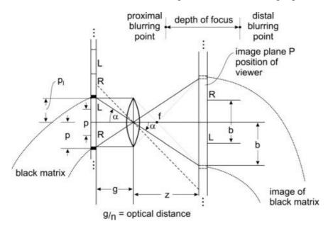
Notice there is some magnification of the pixel pitch p into a larger image pitch b on the image plane, that should be ideally corresponding with the interocular distance, which is 65 mm on average. This magnification is given by:
