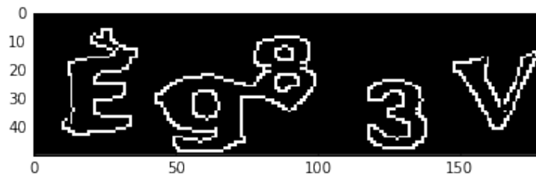
Figure 3.6: Effect of the Canny edge detection algorithm
