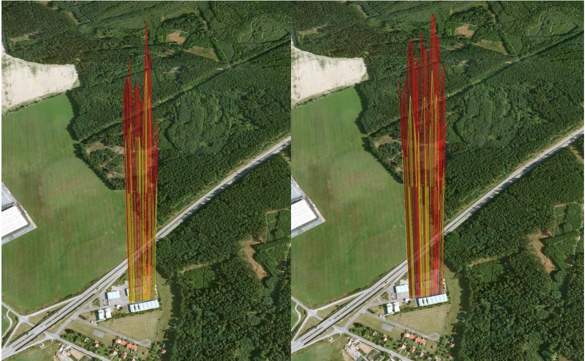
Fig. 26 - RSSI in case of sender switched off (left) and switched on (right)
