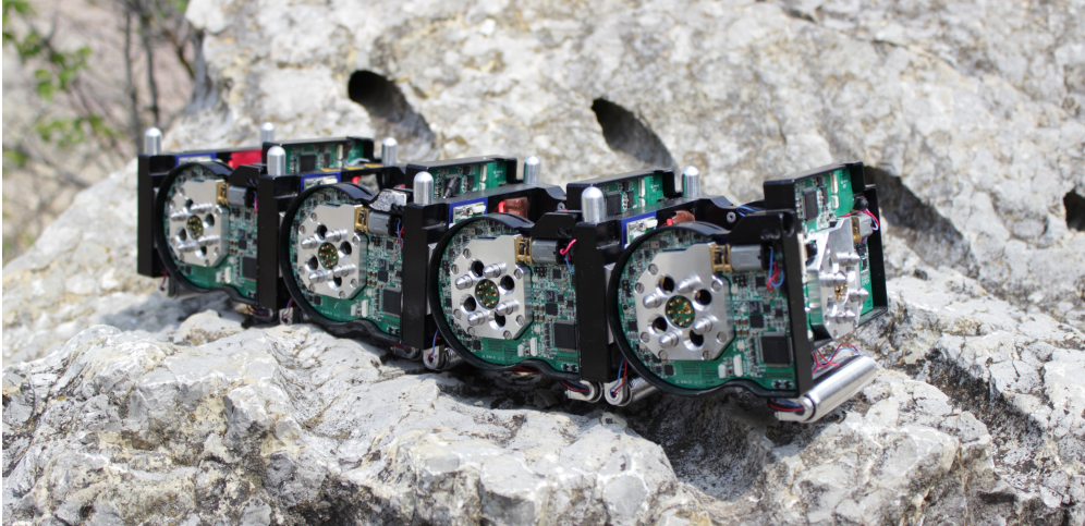
FIGURE 1.2: Example of Snake-Like construction of CoSMO modular robot.
