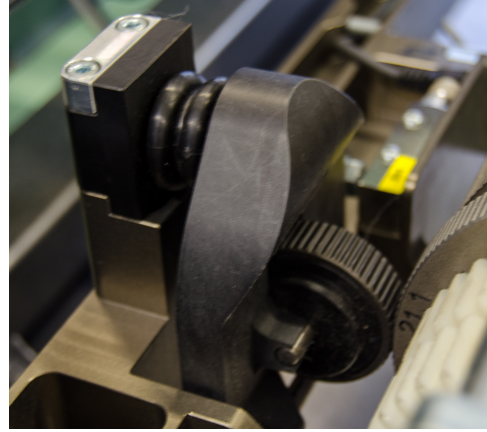
(b) : Sensor application in a combing machine
