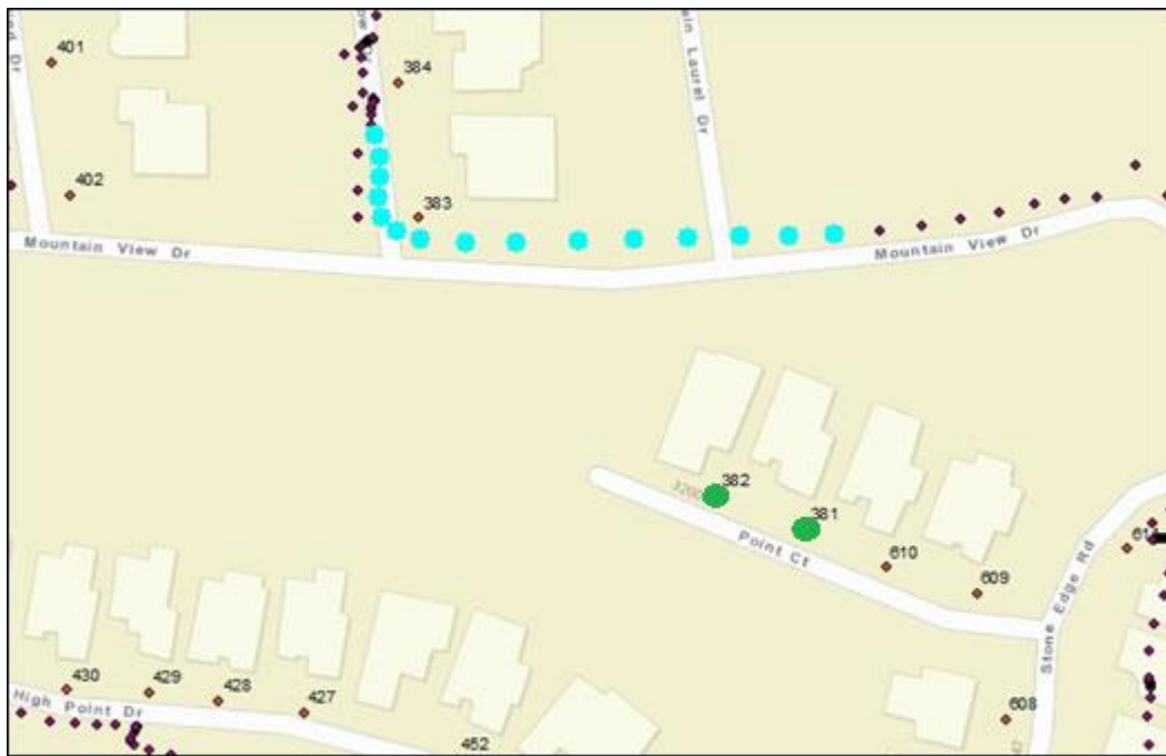
Figure 6.4: Join based on spatial location error, (Purple points – path report logs, red points – container position, green points – incorrectly assigned bins, blue points – path report logs that caused incorrect assignment.)
