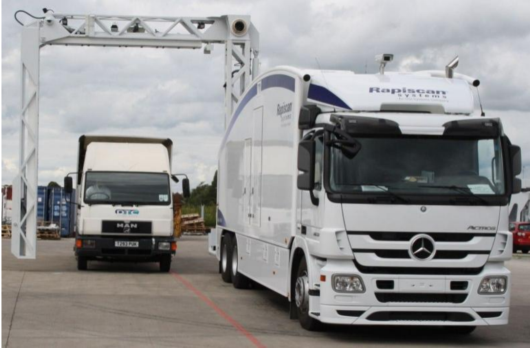
Figure 2.3: Mobile NII Equipment – Rapiscan Eagle M60 (Rapiscan Systems 2014)
