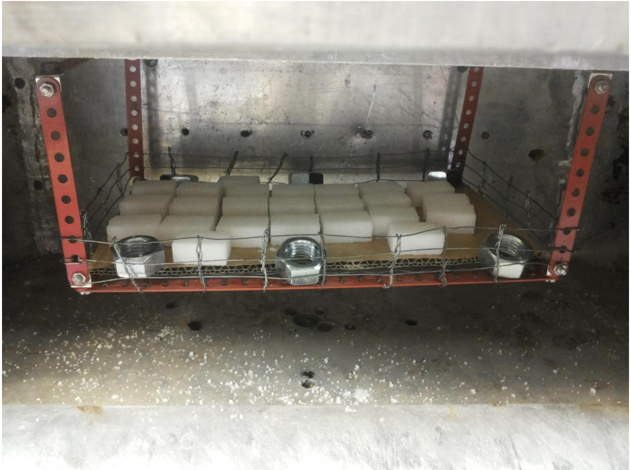
Figure 24. Wet sugar cubes arrangement on drying basket
