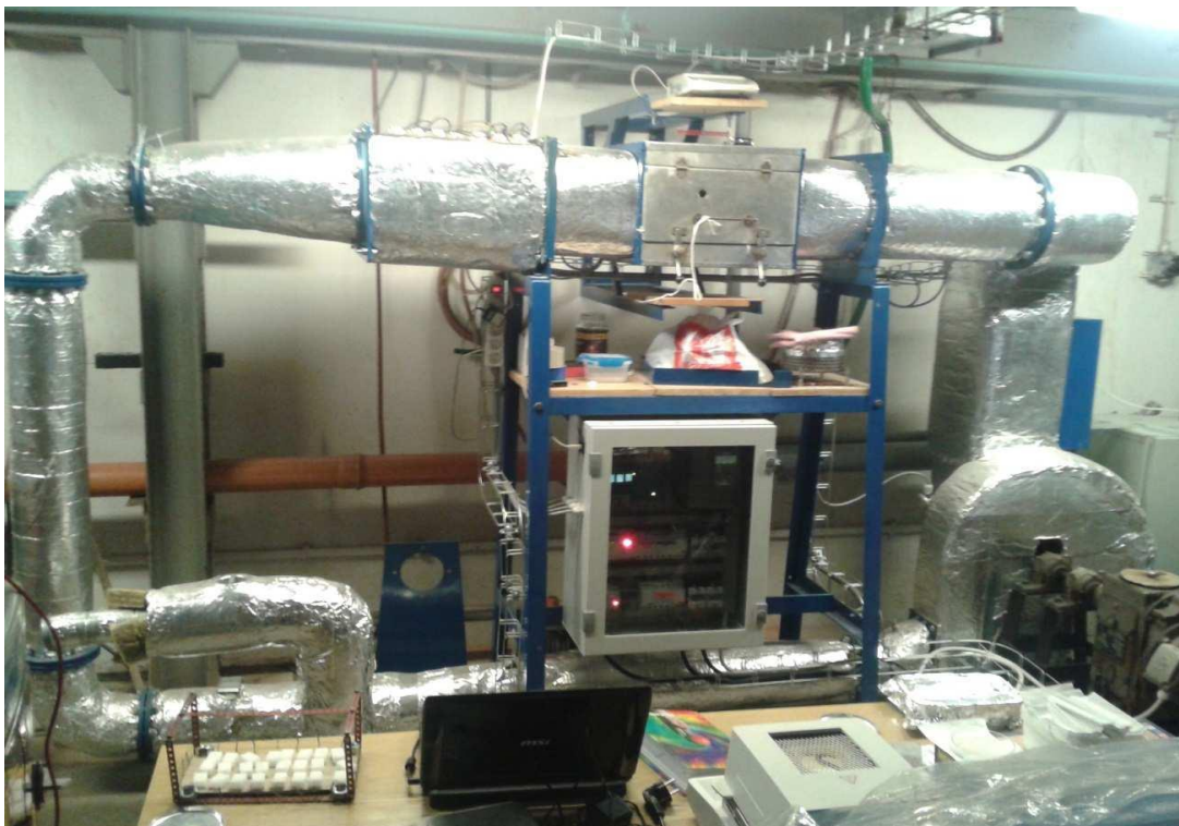
Figure 20. Circulating dryer in the indoor laboratory of the Institute of Process Engineering, Faculty of Mechanical Engineering.
