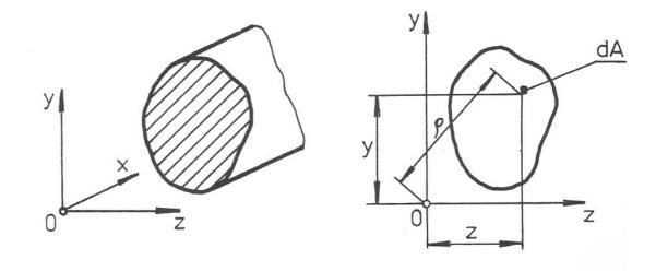
**Figure 2.4:** The beam placed in coordinate system and the plane of the cross section [2] According to the figure 2.4 one removes the element dA = dydz from the cross section *A*, which has the coordinates *y* and *z* relative to the axes *y* and *z*. [2]
