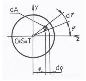
Figure 2.5: The cross section of the circular beam with the cylindrical coordinates [2]
