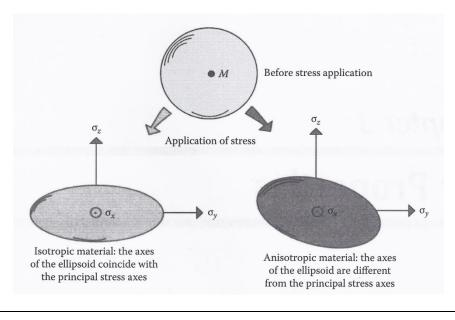
**Figure 1.3:** Schematic of deformation [5]
