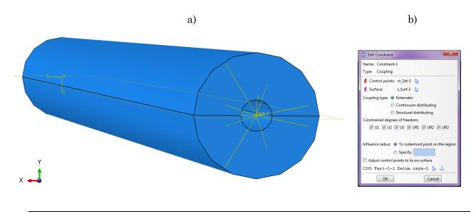
Figure 3.20:a) The pipe with the shown coupling propertiesb) The window for editing the coupling properties
