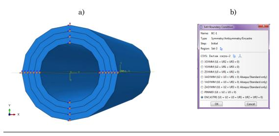
Figure 3.34:a) The beam with shown the fixationb) The window for editing the boundary condition
