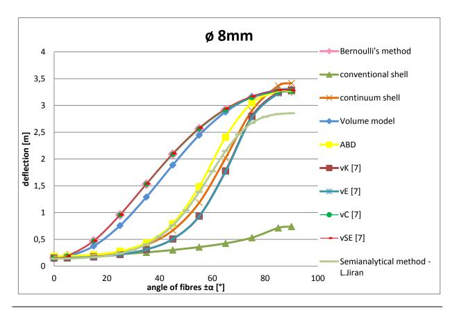
Figure 4.4: The graph of the deflection of the pipe with 8mm inner diameter
