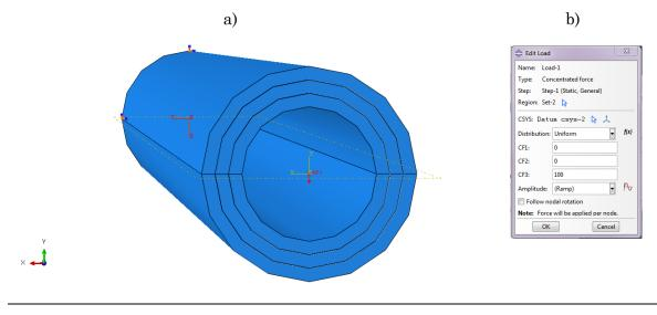
Figure 3.33:a) The pipe with the shown load and the fixationb) The window for editing the load
