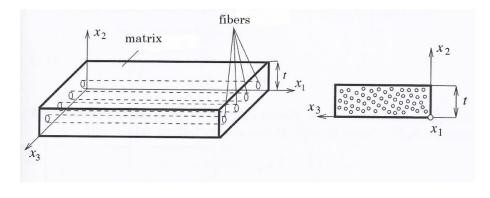
Figure 1.6: An example of the unidirectional composite material [1]
