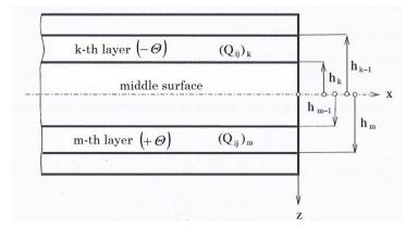
Figure 1.11: Antisymmetric laminate [1]
