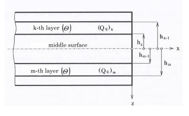
Figure 1.10: Symmetric laminate [1]
