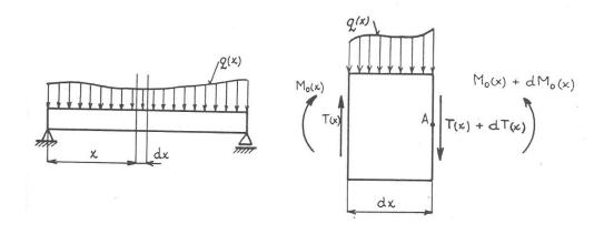
Figure 2.1: Loaded beam and out of joint element with force effects [2]
