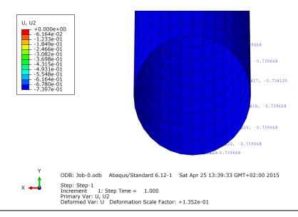
**Figure 3.14:** The detail of the end of the deformed beam with the values of the deflection
