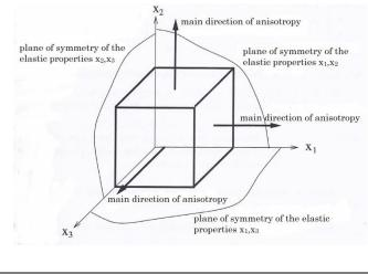
Figure 1.1: Orthotropic material [1]
