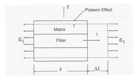
Figure 1.4: RVE subject to longitudinal uniform strain [4]
