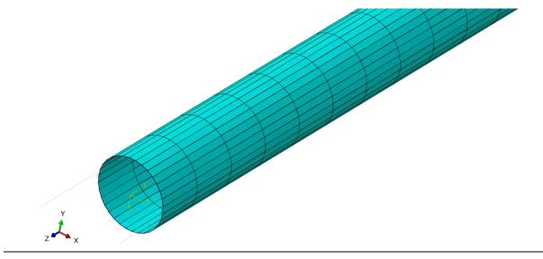
Figure 3.11: The meshed beam
