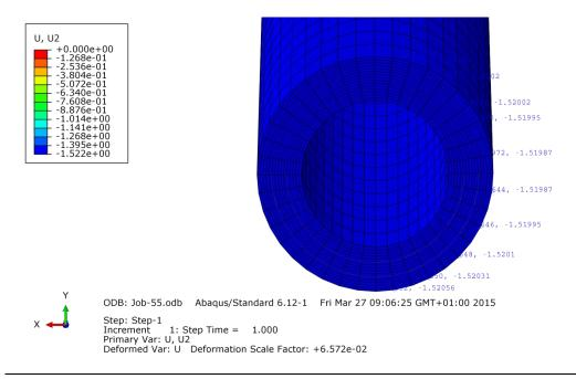
**Figure 3.38:** The detail of the end of the deformed beam with the values of the deflection
