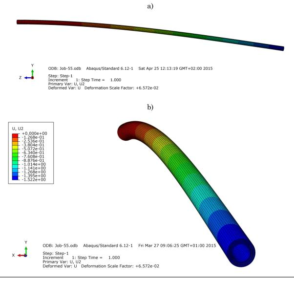
Figure 3.37:a) The deformed beam shown in the yz planeb) The deformed beam in a general perspective with the scale
