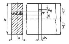
**Figure 2.7:** The cross section of the rectangular beam loaded with shear [2]
