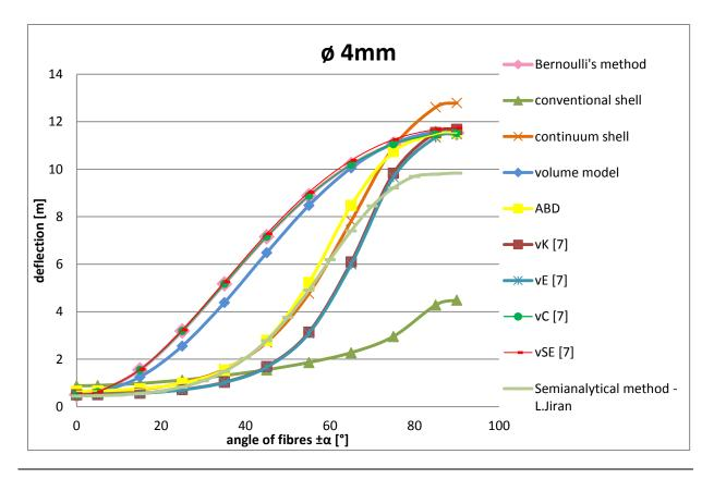
**Figure 4.2:** The graph of the deflection of the pipe with 4mm inner diameter
