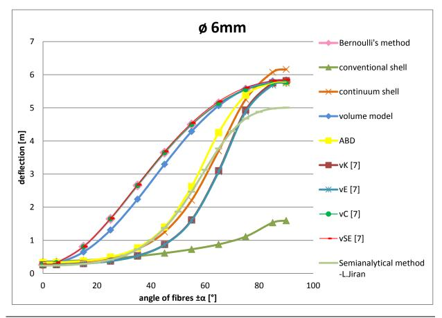
**Figure 4.3:** The graph of the deflection of the pipe with 6mm inner diameter
