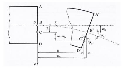
**Figure 1.9:** A part of laminate in the plane *xz* [1]
