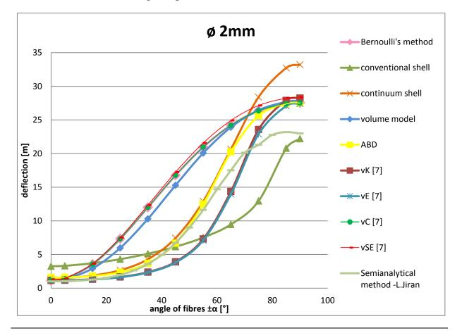
Figure 4.1: The graph of the deflection of the pipe with 2mm inner diameter
