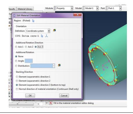
**Figure 3.29:** The window for specify the orientation of the material
