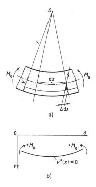
**Figure 2.3:** The part of the beam with marked extension [2]
