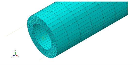
Figure 3.35: The meshed beam
