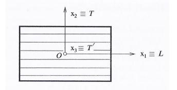
**Figure 1.7:** An example of the unidirectional composite in the coordinate system O(L, T, T') [1]
