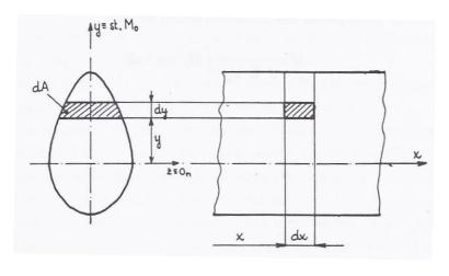
**Figure 2.6:** Cross section of the general beam [2]
