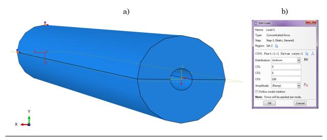
Figure 3.21:a) The pipe with the shown load and the fixationb) The window for editing the load
