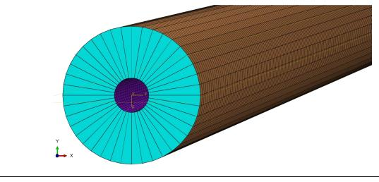
**Figure 3.22:** The meshed beam with the layup orientation
