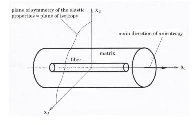
**Figure 1.2:** Transversely isotropic material [1]
