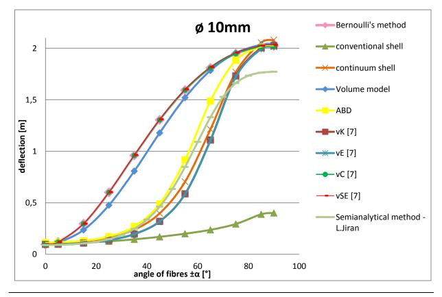
**Figure 4.5:** The graph of the deflection of the pipe with 10mm inner diameter
