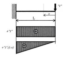
**Figure 3.2:** The beam loaded by the unit force with the course of the shear force and of the bending moment [3]
