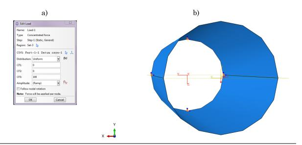
Figure 3.9: a) The window for editing the load b) The pipe with the shown load and the fixation
