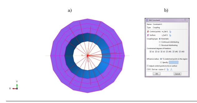
Figure 3.32:a) The pipe with the shown coupling propertiesb) The window for editing the coupling properties
