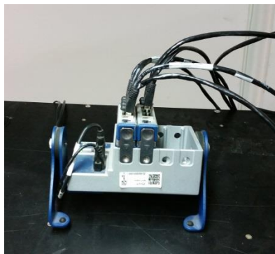
Fig. 5-5 Measuring modules and NI CompactDAQ4-Slot USB Chassis
