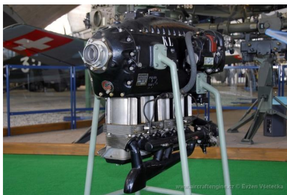
Obr.č.4 motor HIRT HM 504 A-2 [7]
