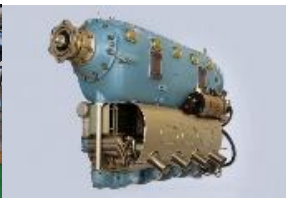
Obr.č.5 motor LOM M132AK [6]
