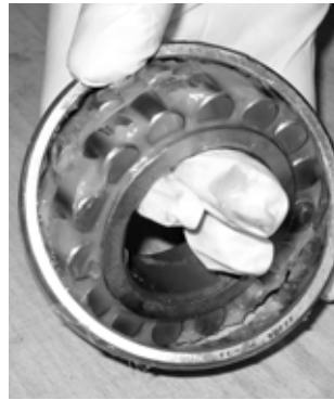
Fig. 21. Grease can easily be packed by hand.
