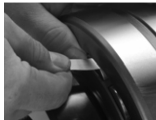
Fig. 14. Measure RIC before installation.
