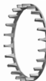
Fig. 9. Split, machined-brass, land-riding, finger-type cage.
