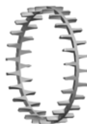
Fig. 7. One-piece, machined-brass, roller-riding, finger-type cage.
