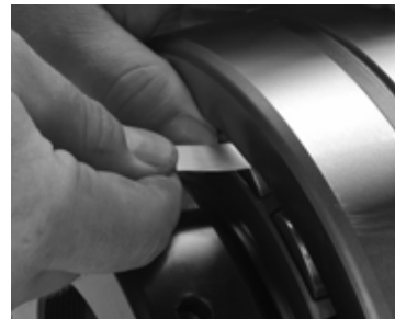
Fig. 18. Measure RIC before installation.
