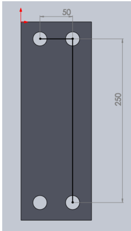
Figure 22 (Dimensions of heat exchanger cover)
