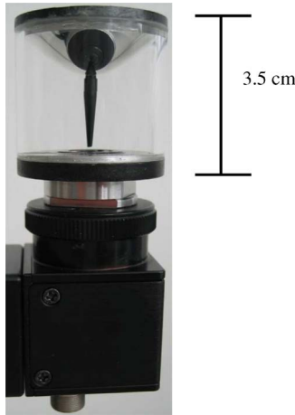
Fig. 2. Catadioptric camera as a combination of lenses and mirrors. The black needle in the middle prevents internal reflections [3].
