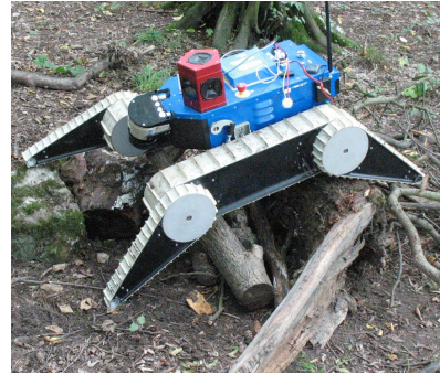
Fig. 1. Adaptive traversability: Robot configuration of the 4 flippers (subtracks) and their compliance is controlled autonomously in order to adapt to the terrain and traverse it in an optimal way. The robot is equipped with rotating laser scanner SICK LMS-151, Ladybug 3 omniscam, Xsens MTi-G IMU, and independent flipper stiffness control for each subtrack.
