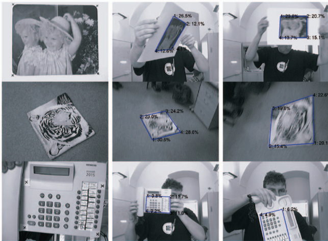
Fig. 14. Ground-truthed sequences. The left column shows images used for training. The middle and right columns demonstrate some successfully tracked frames with strong motion blur from the testing sequences. A blue rectangle delineates the object. Percentage values in corners are current corner speeds related to the current size of the object upper edge.
