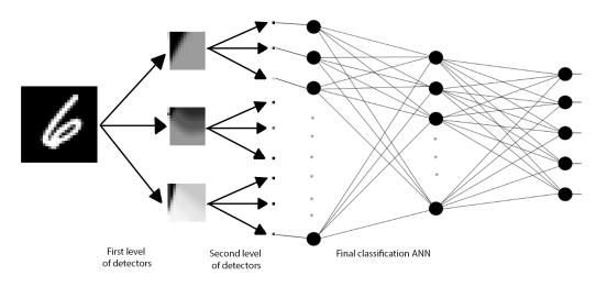
**Figure 3.8.** The illustration of the tree like architecture. The first level contains three detectors, where each of them transform original images into a space of 14x14 pixel images. The second level contain three detectors for each transformed image space of previous layer. The second level detectors transform the images into single value outputs. At the end a final ANN combine all outputs of the second level together and train itself on them by RProp.
