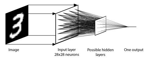
Figure 3.1. The illustration of the detector. Each pixel of the image has corresponding input neuron. There can be zero or more hidden layers and all layers are fully connected to adjacent ones. The output is only one value.
