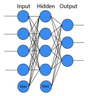
Figure 2.2. The ANN is a system of interconnected neurons, similar as in the human brain. Each circular node represent neuron and each line represent connection. In each layer can be found a bias neuron, which is always active.
