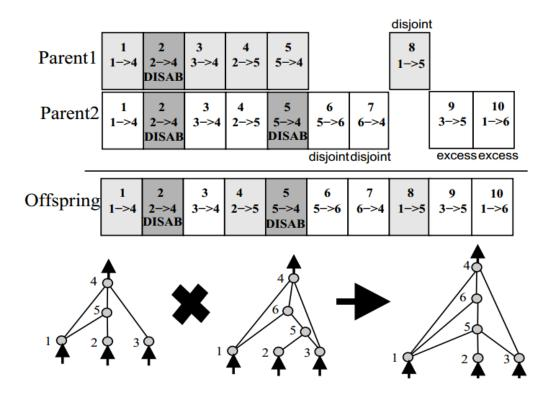
Figure 2.6. Example of the crossover in the NEAT algorithm. Matching up genomes for different network topologies using the innovation numbers. In this example the same fitness for both parents is assumed, therefore offspring gets excess and disjoint genes from both parents. Source: [18]
