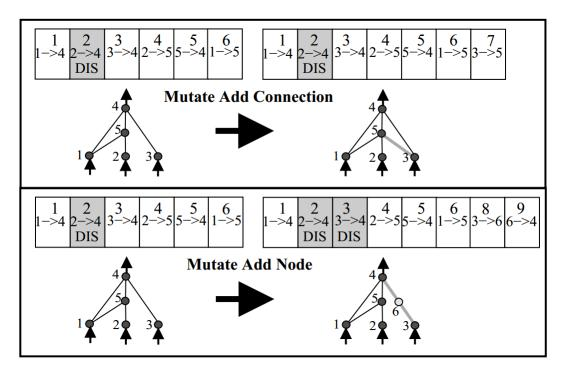
Figure 2.5. The two types of structural mutation in NEAT. Both types, adding a connection and adding a node, are illustrated with the connection genes of a network shown above their phenotypes. Source: [18]
