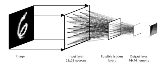
**Figure 3.7.** The complex detector transforming MNIST images into 14x14 pixels image. It has input layer of 28x28 neurons, possible hidden layers and output layer of 14x14 neurons.
