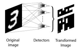
**Figure 3.5.** The illustration of the approach creating grid with rows and columns depending on the class. It takes 100 detectors and order their outputs into a grid. You can notice that all detectors int the row corresponding to number three and most of the detectors from the column corresponding to number 3 are activated in the transformed image.
