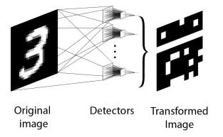
Figure 3.4. The illustration of the approach creating grid with rows depending on the class. It takes 100 detectors and order their outputs into the grid. You can notice that all detectors in the row that correspond to the number three are activated in the transformed image.
