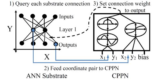
**Figure 2.7.** A CPPN describes connectivity. The ANN substrate has assigned coordinates. Step 1: Every connection between the neurons in the substrate is queried by the CPPN to determine its weight. Step 2: For each such query, the CPPN inputs the coordinates of the two neurons, which are highlighted in the substrate. Step 3: The weight between them is the output by the CPPN. Source: [4]
