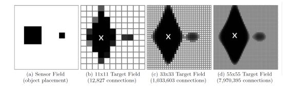
**Figure 2.8.** Activation Patterns of the same CPPN with different rescaling. The placements of the objects for this example are shown in (a). Each square represents a neuron in the target field. A darker color signifies higher activation and a white X denotes the point of the highest activation, which is correctly at the center of the large object in (a). Source: [1]
