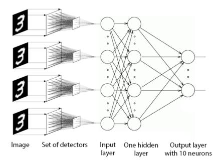
Figure 3.2. Complete structure used for image recognition. First each detector transform image into one value output, then following ANN classify image based on outputs of detectors.
