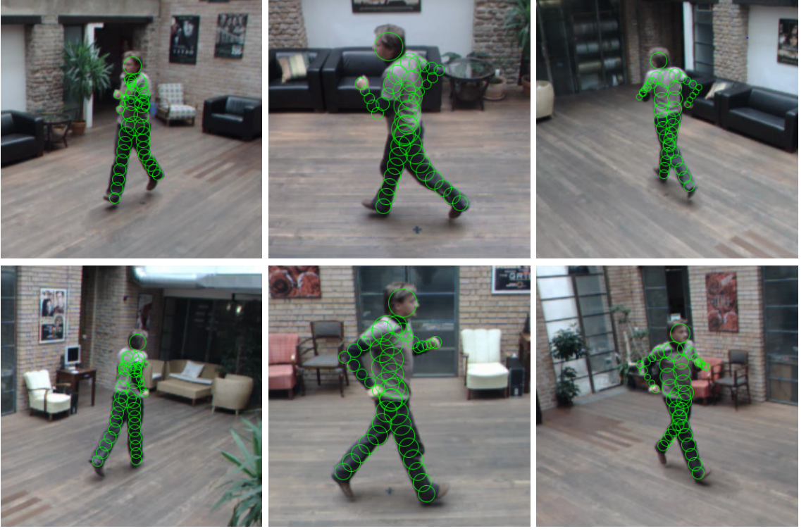
Figure 2.4: Projection of the body model to 6 different camera images using the (2.6) formula. Note that only crops from the whole images are shown here for better detail.
