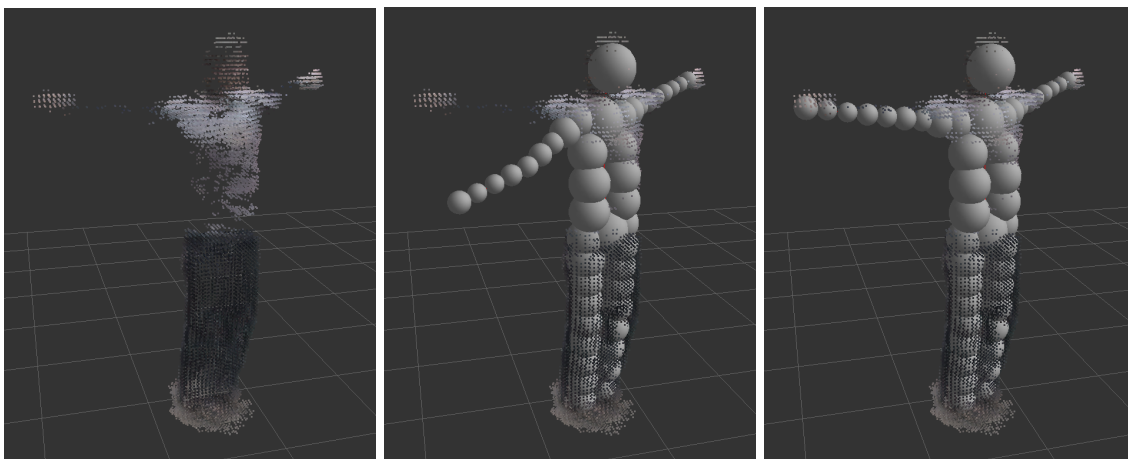
Figure 4.2: Setting the initial solution for the first frame. Helper point cloud (left) moving the model's arm via inverse kinematics (middle) initial solution and the point cloud (right)
