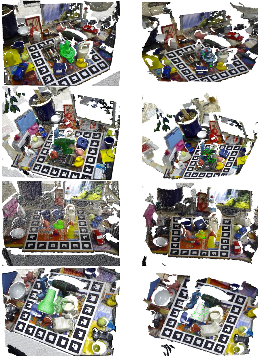
Figure 34: Examples of the detected objects in Hinterstoisser's dataset. Coloured point clouds of each scene with detected object in green colour are shown in the left column. The points in the scene which voted for that particular object pose are shown in the right column. The red circles denote the reference points and the green ones the paired scene points.
