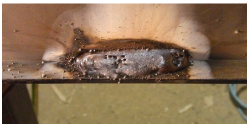
Fig. 28. SMAW weld with the slag
