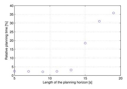
Figure 5.12: Results of the Planning Horizon Test. With longer planning horizon, the algorithm has to search larger portion of the planning space. With the planning horizon longer than 20 seconds, the simulator ran out resources.
