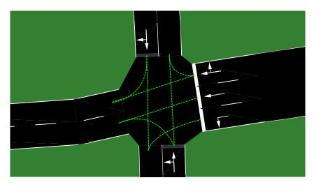
Figure 3.1: Junction as represented by SUMO. The green dashed lines represent connections from the incoming lanes to the outgoing ones. The visualization is exported from the graphical user interface of the SUMO toolkit.
