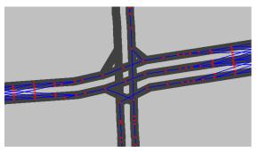
(a) Discretization of the SUMO road network. The discretization factor is set to a large value, i.e. number of metres.
