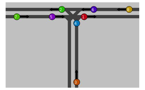
Figure 5.7: Situation after the start of the simulation. Lower number means higher priority. The vehicle number 4 has higher priority than vehicles 6 and 5, so they must slow down and let the vehicle 4 pass.
