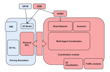
Figure 5.1: Architecture of the AgentDrive platform. The core parts are depicted in red. If the external simulator is connected, the blue modules are also used.
