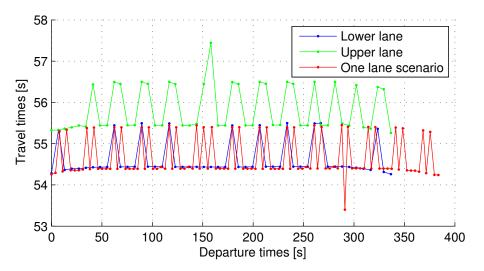
Figure 5.4: Plot illustrating the travel times for each vehicle. The blue and green lines are from the two-lane scenario, whereas the red line is the scenario with single lane. Note that the points are connected with lines only for more readability.
