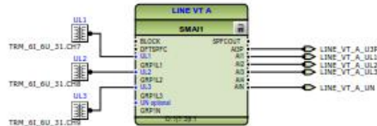
VOLTAGE CIRCUITS LINE VT CIRCUIT "A" FOR DISTANCE PROTECTION AND FUSE FAIL
