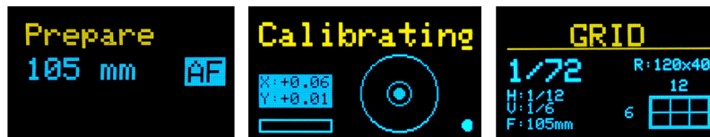
Figure 33: Display with three screens. Left image shows co-called pre-grid mode which runs before grid process starts and shows actual focal length and focus mode. Central image shows calibration mode allowing set the head to the correct position. The right image is the screen of the progress on grid mode.
