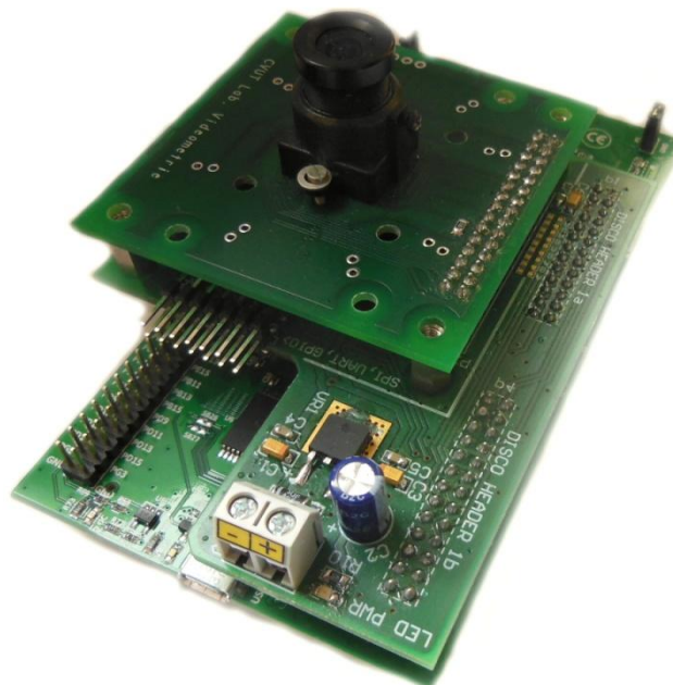
Fig. 9 - CONN.BOARD F429 for CMOS module and STM32F429I-Disco kit connection
