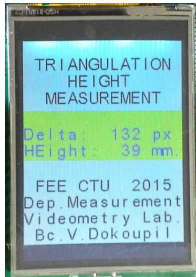
Fig. 39 - STM32F429I-Disco display for the laser height measurement application
