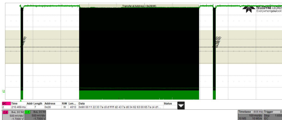
Fig. 8.16: Analysed communication with PCap02A - Write to SRAM
