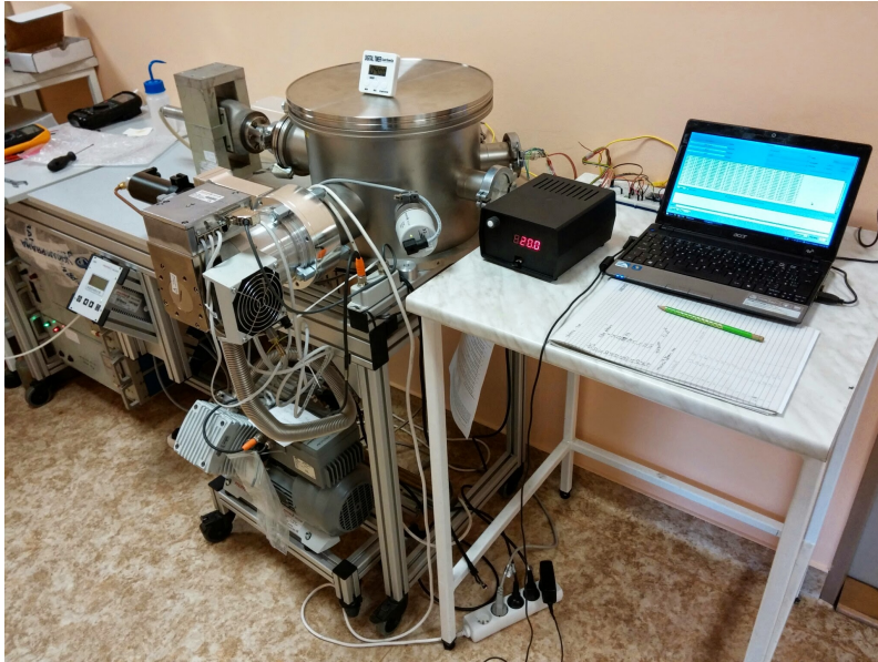
Fig. 10.8: Arrangement of Vacuum test
