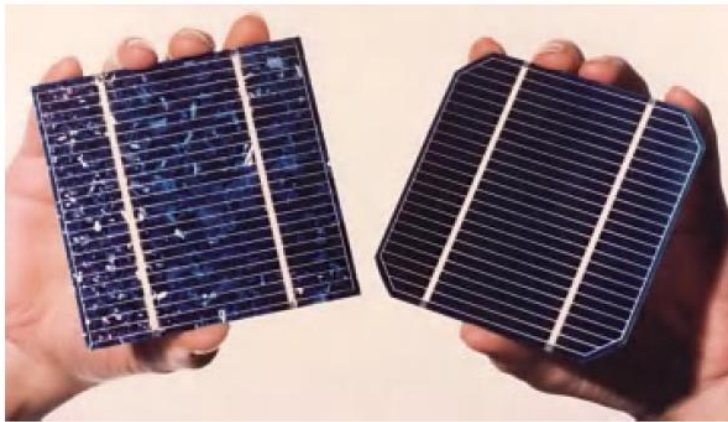
Figure 2: Left - polycrystalline solar cell, right - monocrystalline solar cell [3].
