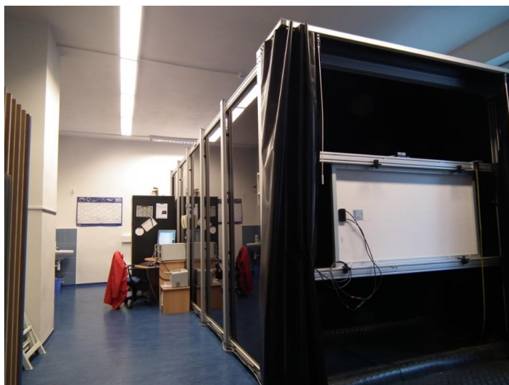
Figure 37: The flash tester was used for our measurements.
