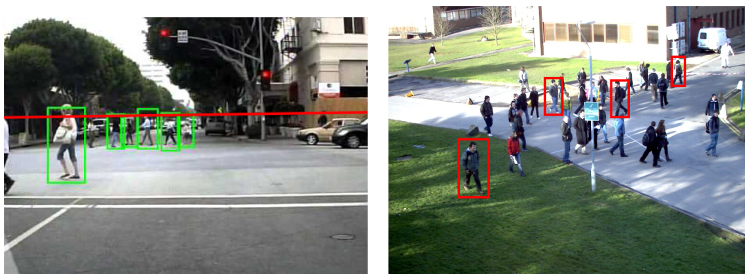
Figure 6 Illustration of the influence of the camera position on the predictability of position and size in various parts of the image. Heads are on the horizon for a car/person view and the size can vary (left). Size can be predicted for each part of the image when overhead camera view is used (right).
