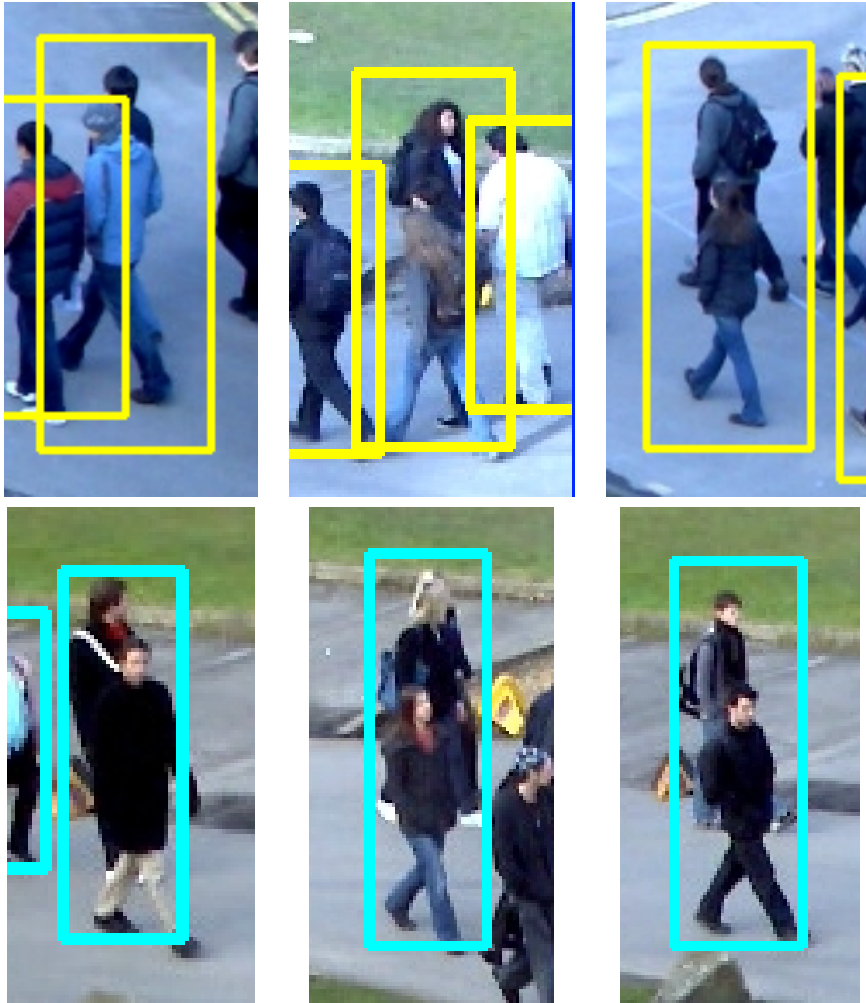
Figure 15 Examples of fault detections produced by person detectors when presented with images containing frequent occlusion. Two people behind each other are detected as a "double person".
