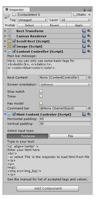
Figure 3.4: The inspector window of a content created from the ContentHtml prefab in the Assets/Resources/ContentPrefab project folder.
