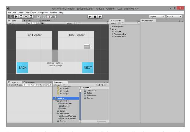
Figure 3.1: The interface of Unity after opening the RadApp project. Note that some of the window components can be relocated, or hidden. Look for the names of the tabs, and by dragging them you can relocate them to match the picture.
