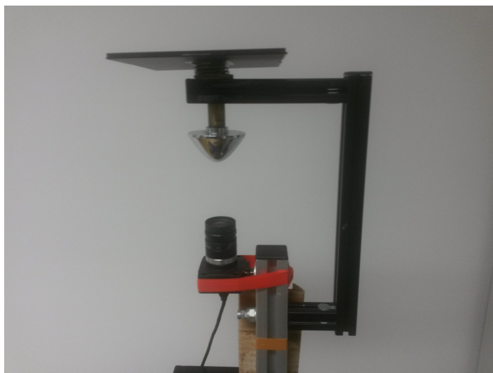
Figure 5: Camera installed on the ATR V mini robot, used for capturing omnidirectional images.
