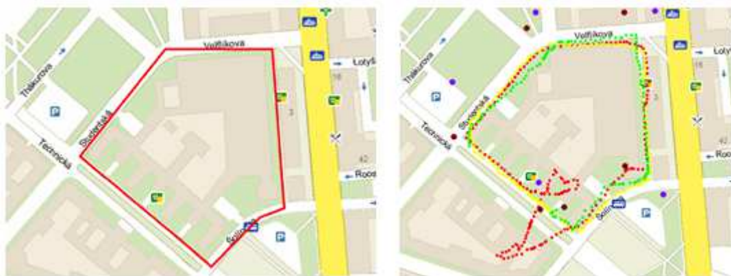
Figure 10.1 Illustration of errors in GNSS positioning in urban canyon
