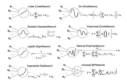
Figure 2.7: Different types of neurons - building blocks of the GAME artificial neural network. Source [63].
