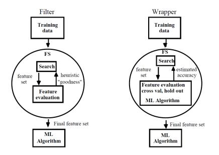
Figure 2.3: Filter and Wrapper feature selectors. Picture published in [40].
