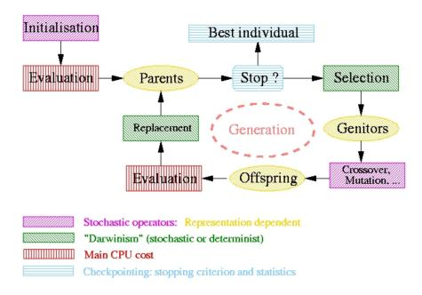
Figure 2.8: Gereral evolutionary algorithm scheme. Source [69].
