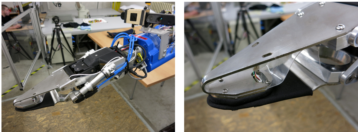
Figure 2: Left: The CloPeMa hand with variable stiffness and tactile sensor. Right: Detail of the hand tip with the tactile sensor.
