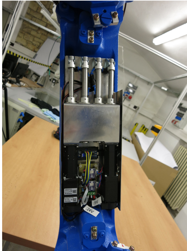
Figure 3: Gripper hydraulics controller box.
