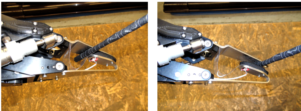
Figure 43: Left: The pole caught inside the gripper. Right: The pole caught well.
