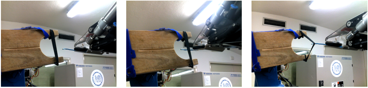
Figure 22: Left: Shooting position. Middle: Loaded. Right: Ready to fire.
