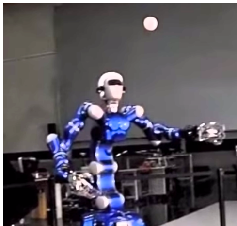
Figure 10: The Rollin' Justin Robot catching a ball.
