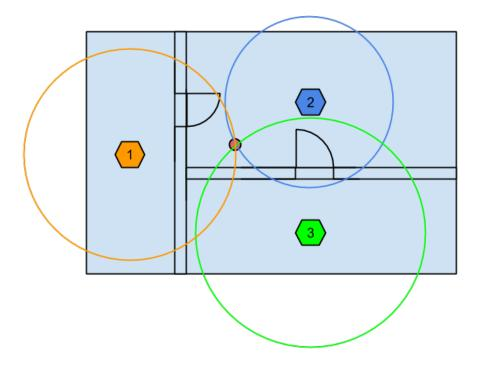
Figure 4.1. Demonstration of trilateration principle. Points 1, 2 and 3 are BLE APs which measure RSSI.
