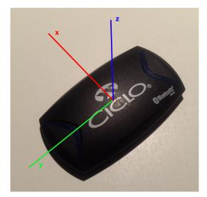
Figure 4.2. Ciclosport heartbeat sensor used for measurements.
