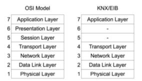
Figure 2.1. Comparation of OSI and KNX layers, [3]
