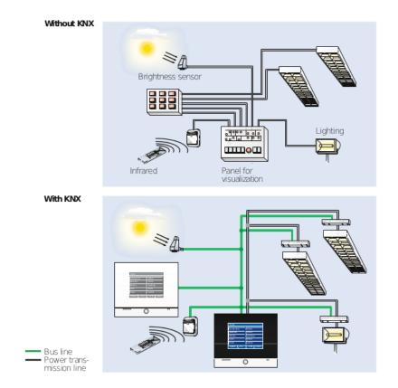
Figure 2.2. Differences between normal and KNX installation, [2]
