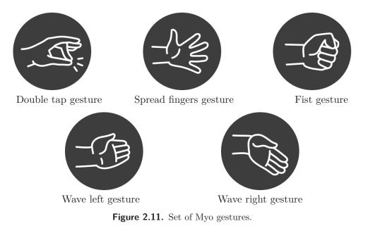
To prevent the misclassification of hand movements as gesture, Myo has a locking mechanism. The mechanism keeps Myo in stand-by mode waiting for only one gesture — Double tap gesture — all other gestures are ignored. When the unlocking gesture is made, Myo starts to look for other hand gestures for few seconds. If, in this period, no
