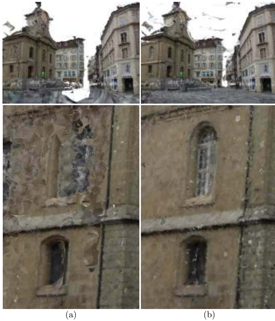
Figure 7.12.: Results for the 'strecha' data set. (a) result of the our implementation of the base-line method textured, (b) result using our method, textured. The weakly supported ground plane is preserved using our method and other surfaces are also constructed better.
