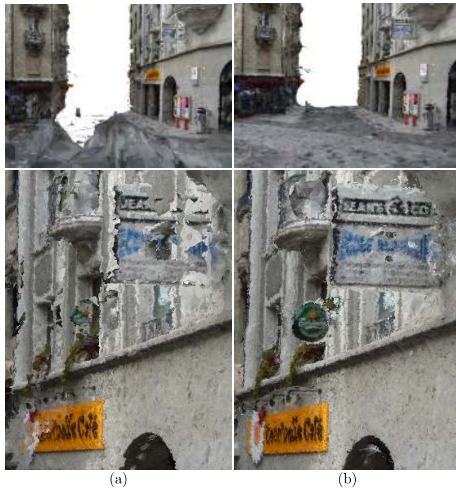
Figure 7.10.: Results for the 'strecha' data set. (a) reconstruction using our implementation of the base-line approach, (b) reconstruction using our approach. Weakly-supported surfaces are better reconstructed using our approach than by base-line approach.
