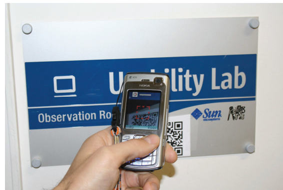
Fig. 3: QR code on a name plate being recognized by camera of smartphone.
