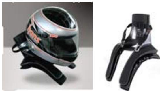
fig 13 - Hans - Restraining extra device is designed for specific seatback angle. For purpose of adjustable seat would this device need additional mechanism development.
