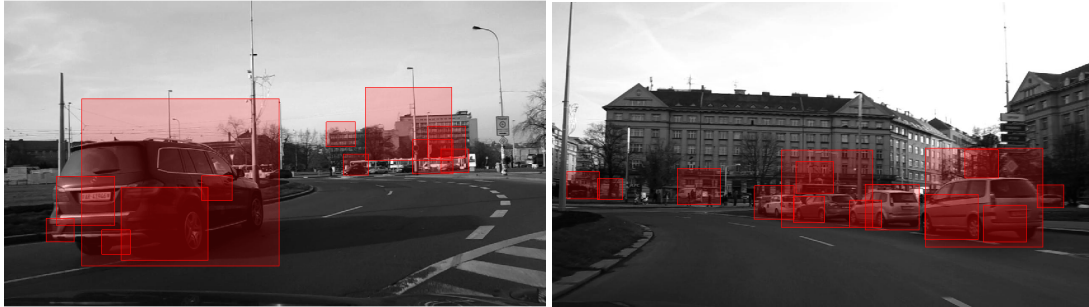
b) LSD window pruning. 1 line within a window required.
