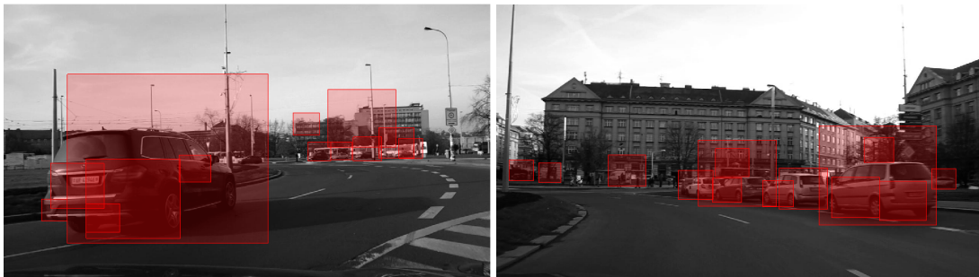
c) LSD window pruning. 2 lines within a window required.
