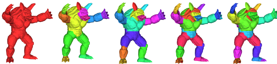
Figure 5.1. Segmentation of a shape with different values of the number_of_clusters variable (1, 3, 5, 7 and 9 from left to right). The smoothing_lambda was set to the value used – 0.15.
