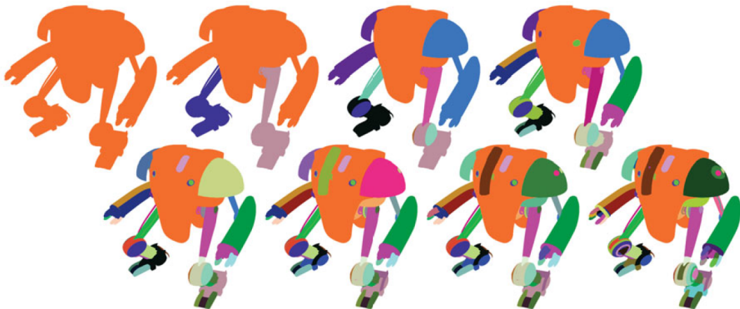
Figure 2.3. An illustration of the hierarchy creation. The coarsest level of the hierarchy is shown top left, the initial part segmentation at the bottom right. Image taken from [Jain et al. 2012].
