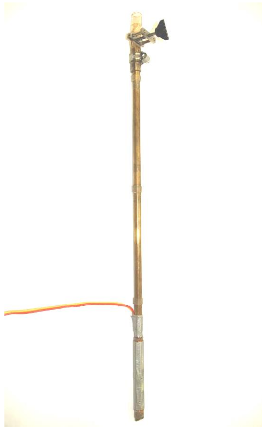
Fig. 7.33 Experimental heat pipe with magnetic plug inside
