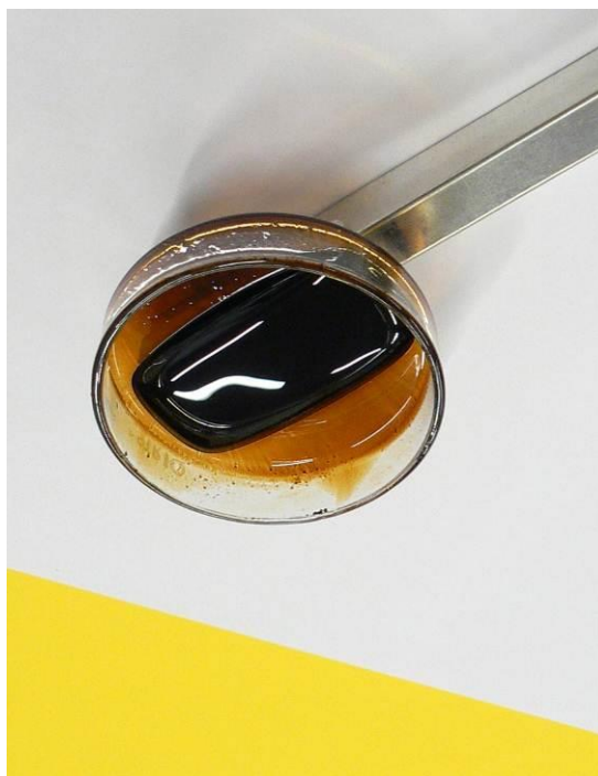
Fig. 6.8 Oil ferrofluid hangs under permanent magnet
