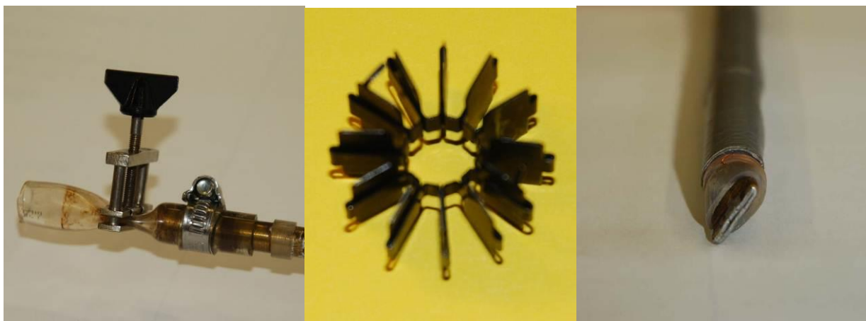
Fig. 7.3 The condenser end with a rubber extension and a clamp; fin radiator optionally placed on the condenser region; the evaporator end
