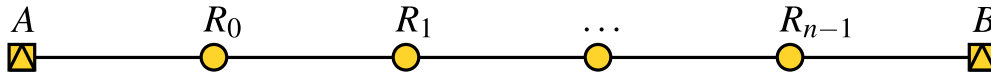
Figure 2.16: Chain topology. Node A bidirectionally communicates with node B via serially concatenated chain of n -relays.
