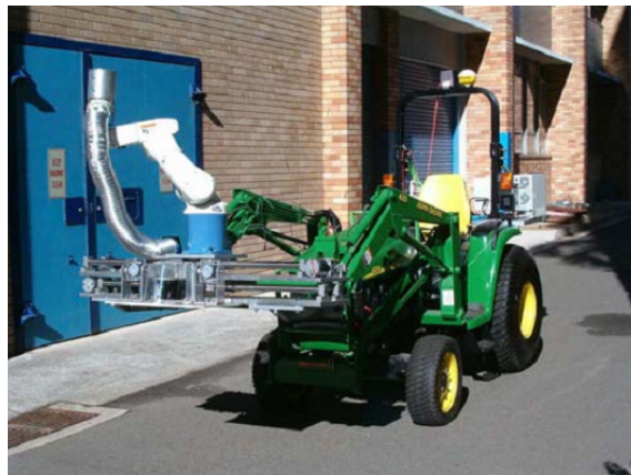
Figure 17. Automatic fruit picking system proposed by Zhao et al. (Source [10])
